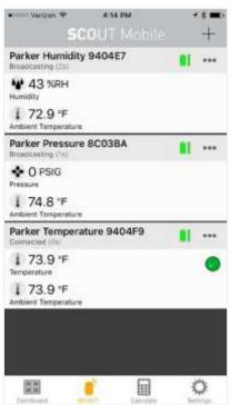
One touch access to sensors that have been added to your mobile device with their latest measurements, alarm status, and sensor mode - broadcasting or connected
