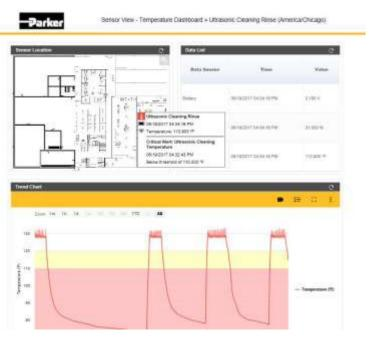
The Asset level dashboard displays live measurements, historical trend chart, and identifying image of your selected sensors attached to a specific asset.
