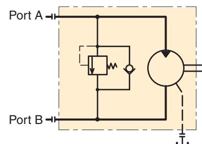
**Diagram for PLC082 pressure relief valves integrated in F12-030**
