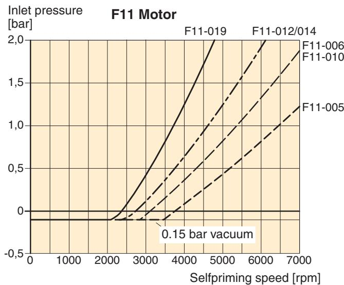
Diagram 1. Min required inlet pressure for Motor.
