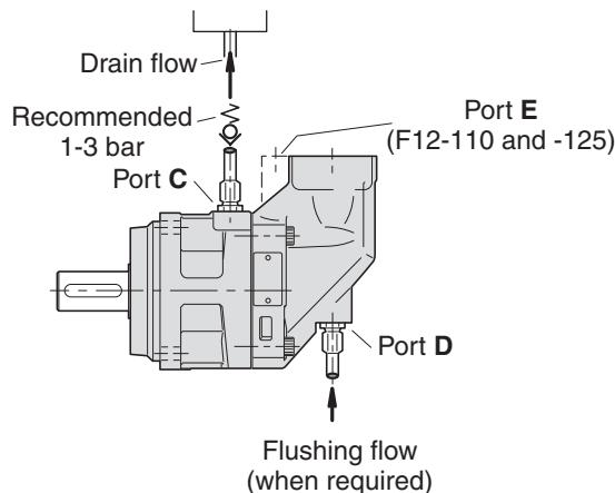
In mounting positions such as 'shaft up' (below) a spring loaded check valve should be installed in the drain line in order to insure a sufficiently high oil level in the case.
