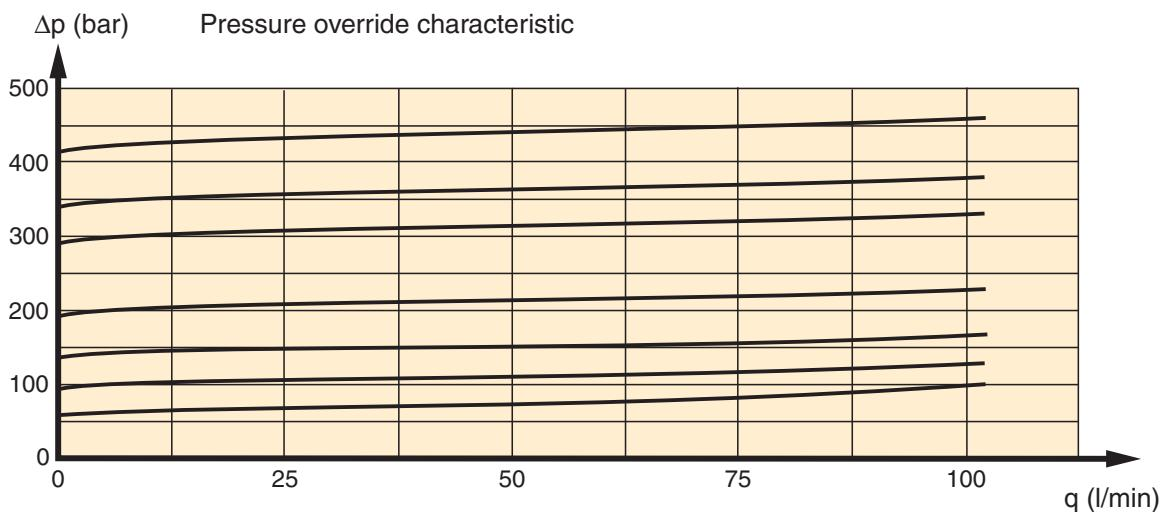
**Diagram for PLC182 pressure relief valves integrated in F12-040 and F12-060**
