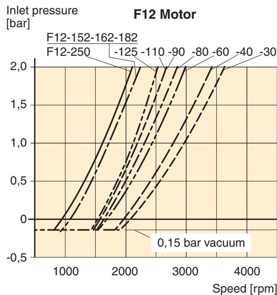
*Diagram 3. Min. required motor (F12-M) inlet pressure.*
