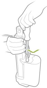
3. Slide the cover onto the actuator.
