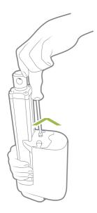
1. Unscrew the cover and remove the two blind plugs.
