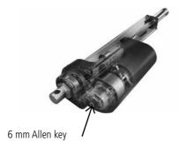
The cover over the Allen key socket must be unscrewed before the Allen key can be inserted and the hand crank operated.
